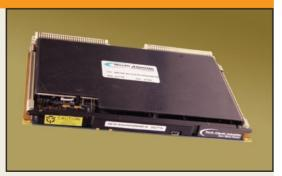
without a VME backplane bus, enabling the board to be used as a stand-alone remote sensor interface without a separate computer board. The 64CS4 operates at -40 °C to +85 °C and 0 °C to +70 °C, and conduction cooling is available.
