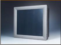
he TPC-120H is an Intel XScale PXA 12.1" SVGA TFT touch panel computer featuring two 10/100BASE-T Ethernet ports. The computer's resolution is 800 x 600, and it comes complete with a Windows CE operating system to support thin-client solutions. I/O includes two RS-232 and one RS-232/485 serial port, two USB 1.1 ports, and one VGA port. The fanless TPC-120H provides one CompactFlash expansion slot and 64 MB SDRAM in a super slim design.
