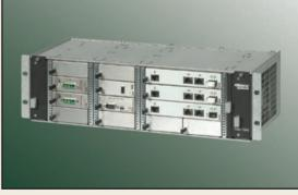
ogy with a fully passive MTCA.0 R1.0 backplane for 10 Gbps throughput. The U-3000's horizontal, flexible design enables installation of double-wide and/or single-wide AdvancedMCs: 4 double-wide and 2 single-wide AdvancedMCs or 10 single-wide AdvancedMCs.
