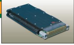
DDR2 memory @ 400 MHz, 128 MB NOR flash, 1 GB NAND flash, and 512 KB NVRAM. I/O includes one XMC/PMC site, two 10/100/1000 Ethernet ports, RS-232 and RS-422 serial channels, and two x4 lane PCI Express egress ports off-board. Its optional 3U VPX I/O expansion companion carrier board, the ExpressReach, provides an XMC/PMC site supporting x8 lane PCI Express port (VITA 42.4) with differential pair I/O routing, along with two x4 PCI Express switch ports to simplify expansion.
